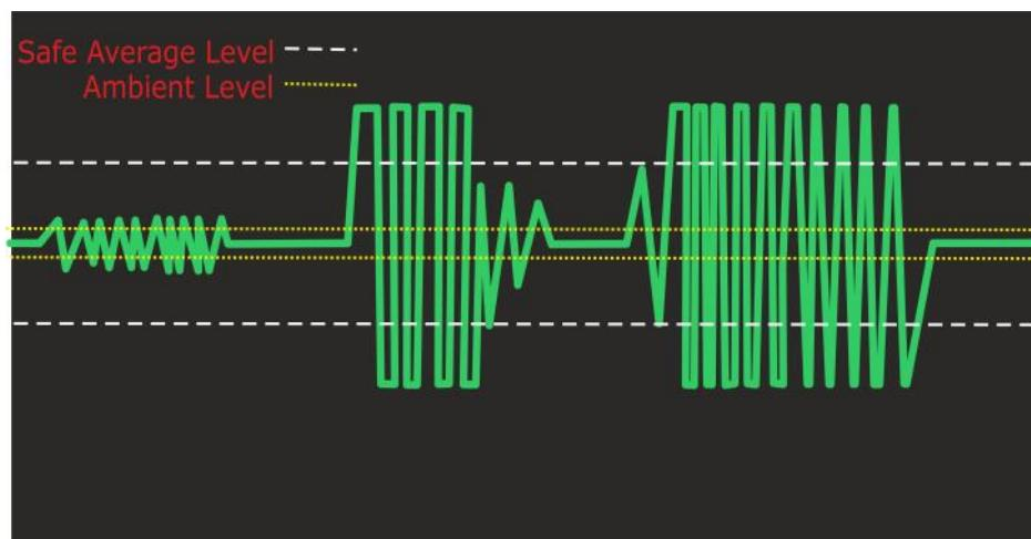
Its significant disadvantage is severe distortion and the relatively poor ability to constrain dose levels, as illustrated by the clipping shown by uniform peaks in diagram 6 (above).
