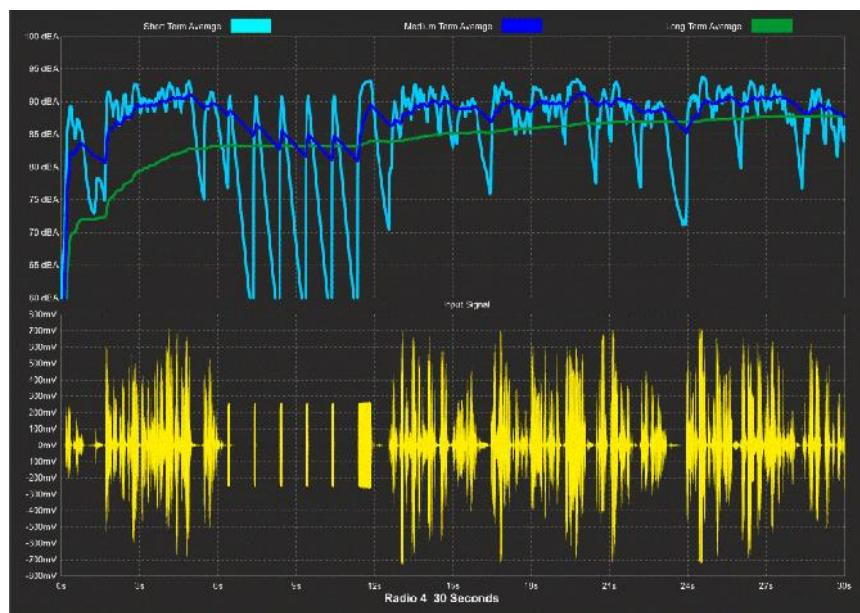
Diagram 2 (below) shows the situation with programme content which has a highly constrained (compressed) dynamic range. A very different picture, but HDM Pro® accurately takes account of what is actually happening at all times. (Radio 1 mix speech and music).
