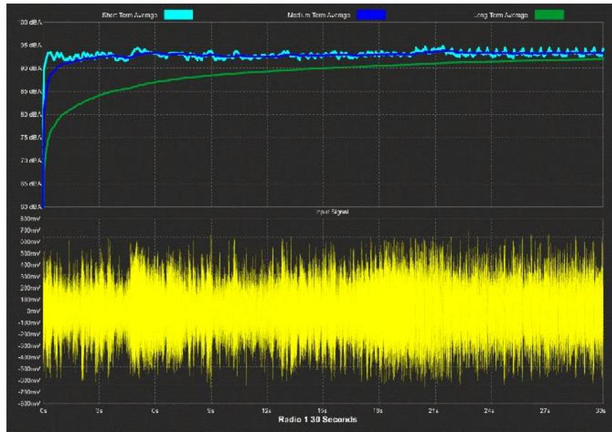
Diagram 3 (below) shows higher quality musical programme content (piano, Radio 3) having a highly variable intensity and wide dynamic range. HDM Pro® has no problem with any amount of channel switching!
