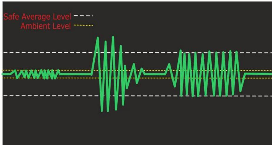
The significant disadvantage (apart from the above guesswork) is that quiet sounds can become inaudible amongst the general ambient sound level, as indicated by the low levels in diagram 5 (above).
